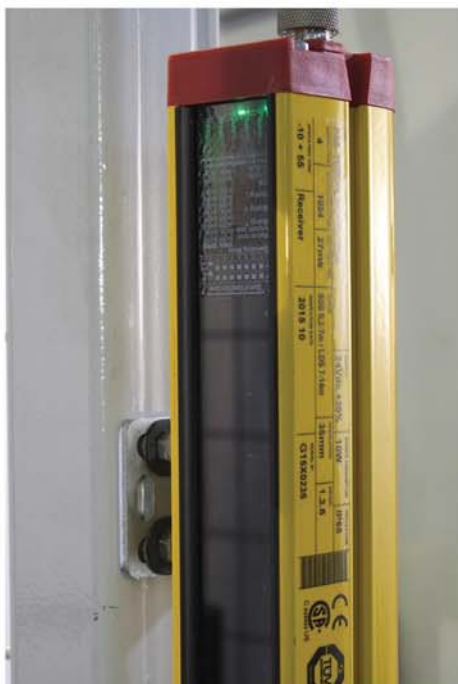
Fig 3 Barreras opticas / Optical barrier
