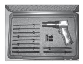
For disassembling the guide valves pneumatically and quickly.
