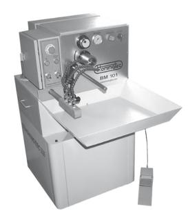
The BM101 Horizontal Honing Machine is an easy-to-use, hand-operated, high-honing precision unit. Due to its compact design and low weight, this honing machine is extremely easy to use. It can be used for honing a wide and diverse rage of diameters ranging between 5 and 100 mm (depending on whether it is machine version A or B), working at spinning speeds from 95 up to 1150 rpm (A or B) according to the diameter of the part to be honed.
