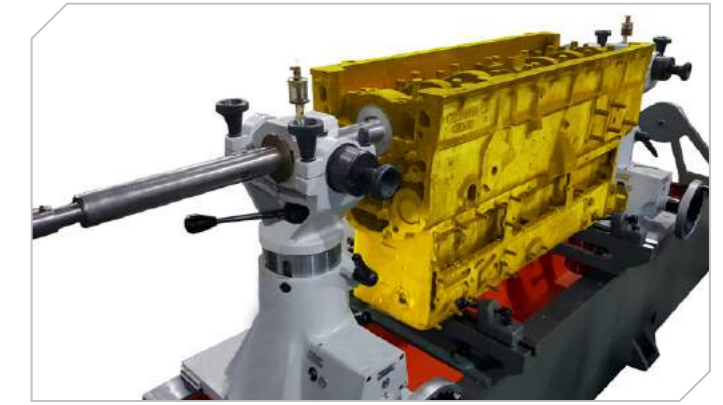
61110 Mil yüksüğü (ekstra) Pivot thimble.Reboring for fitting of oversize bearings (extra)
