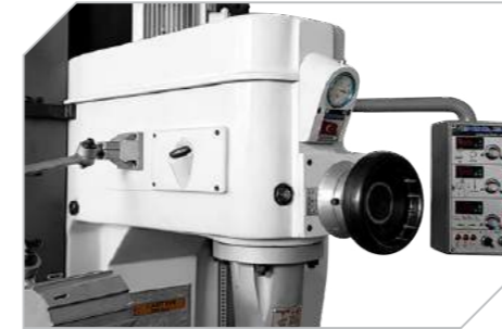
Kontrol panosu ve şanzıman Control panel and transmission
