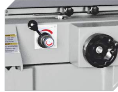
Hidrolik tabla hız ayar kolu Hydraulic table speed adjusting handle
