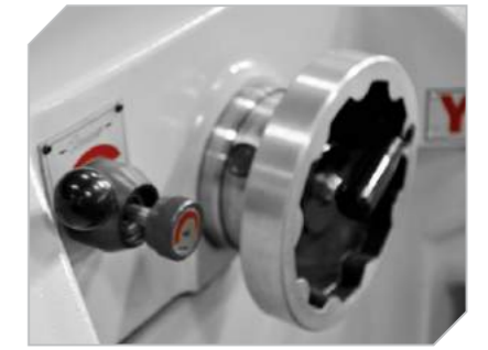
Hidrolik tabla hız ayar kolu Hydraulic table speed adjusting handle
