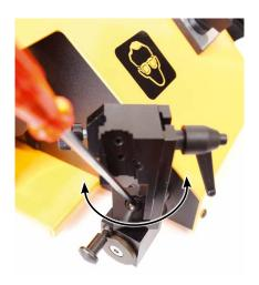
On the standard toolholder are positions for grinding Mira BB turning tools, on all three surfaces.
