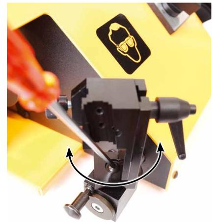
On the standard toolholder are positions for grinding Mira BB turning tools, on all three surfaces.
